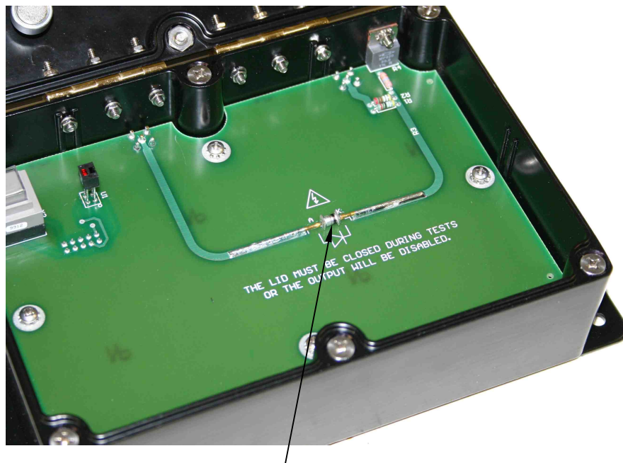
A MELF-packaged Device Under Test (DUT)
